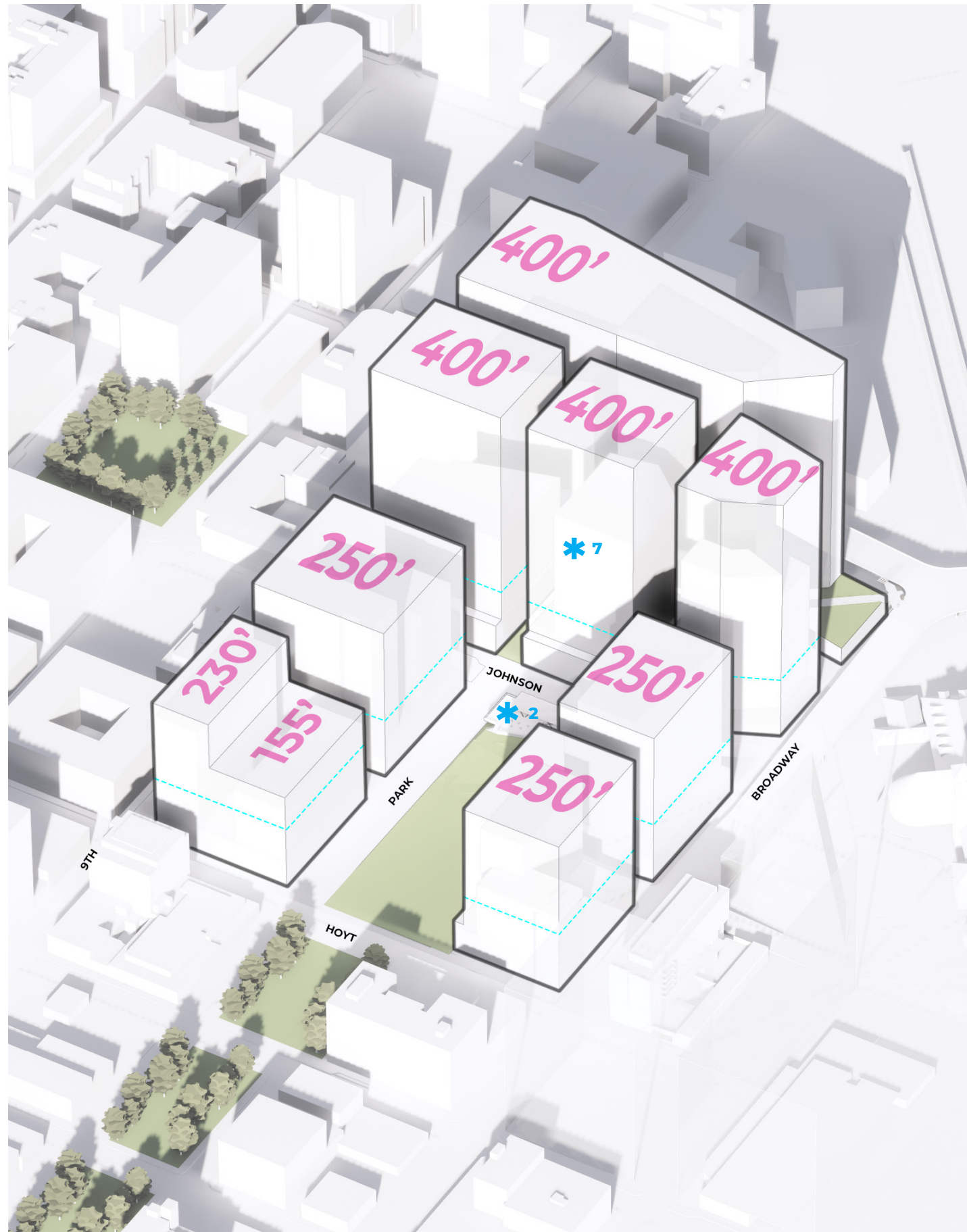
Figure 4.15 Building Envelope - Southwest View
